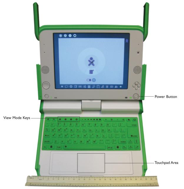
Figure 1. A picture of the XO laptop highlighting various parts of the machine. A ruler at the bottom provides scale.
